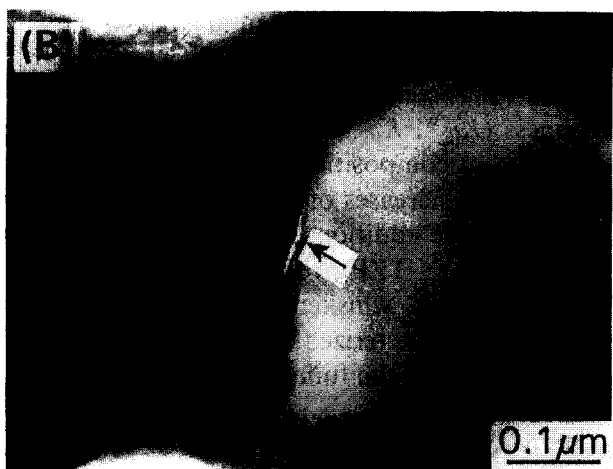
Fig. 6. (A) TEM micrograph of 20 vol% 3Y-TZP/ZrSiO 4 composite. (B) Microcrack in 20 vol% 3Y-TZP/ZrSiO 4 composite.
